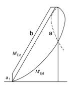
VIS calculates the amplified moment diagrams for slender walls based on the picture above. The tension shift a1 is calculated in accordance with EC8 § 5.4.2.4.
