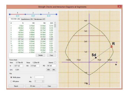
If the design forces are represented by point Sd and the corresponding section strength is represented by point R, where Sd and R are on the same N-M plane, the corresponding D/C value is:
